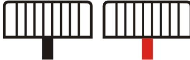
Step 1: Cut from fret leaving whole tab Step 2: Trim tab along straight edge of part
