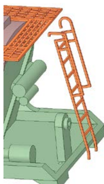
Ladder bent to slope
