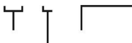
Profiles for Plough (L) and Brake (C) Handwheels and Guard Rails (R)
