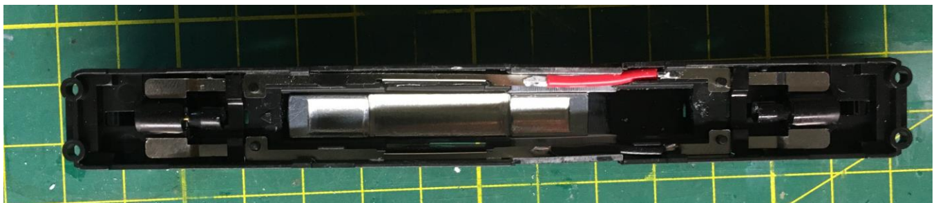
Figure 10 Contact strips reinserted and held in place by retainer pieces, final solder joint of wire to forward portions made inside the extension piece
