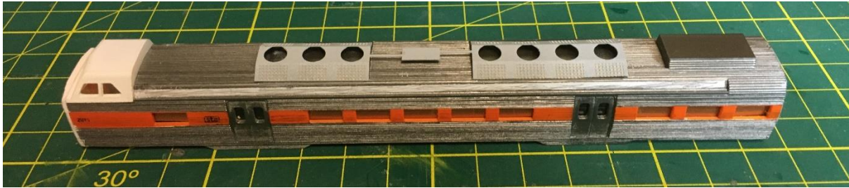
Radiator blocks in place on roof
