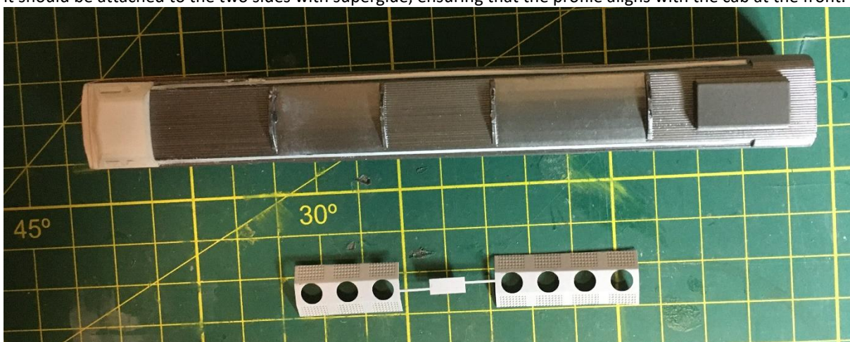
Radiator blocks, folded and painted, prior to attachment
