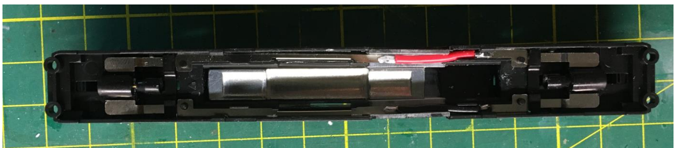
Figure 8 Contact strips reinserted and held in place by retainer pieces, final solder joint of wire to forward portions made inside the extension piece
