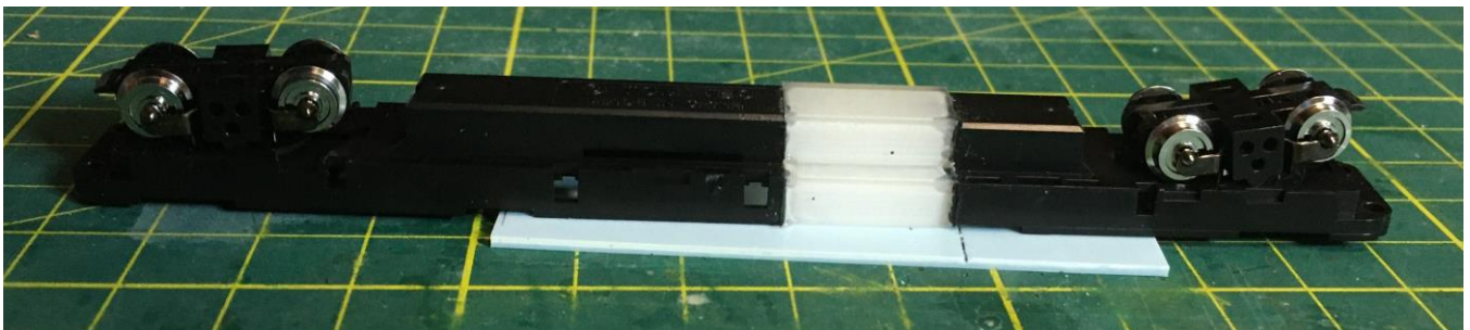
Figure 4 Extension piece glued into chassis halves – note support on 1 mm spacer to clear bogie worm boxes
