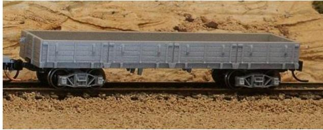
**The Prototype:** A total of 95 bogie wooden open wagons were built for the SAR in 1914-15. Some of these survived into the ANR era and were recoded AOWA. Some even survived and were painted in the AN green and yellow colour scheme. Numbers remaining in 1957 were in the range 3143 – 4049.
