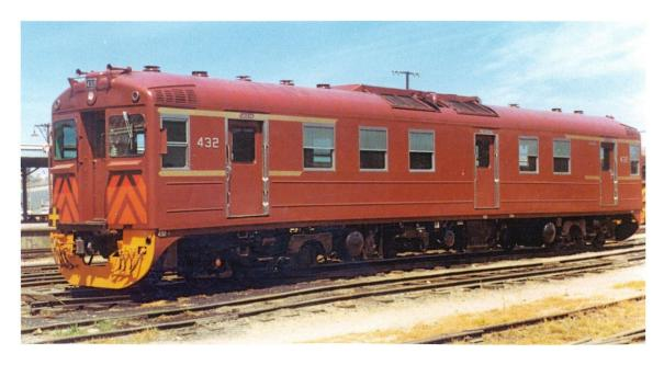
**The Prototype:** New double ended suburban railcars were produced for the SAR from 1959 to 1971 by the Islington workshops to complement the 300 series redhen railcars and add flexibility to the fleet, with the possibility of running single units on lightly patronised services. The double ended cars were numbered in the 400 class (400 - 436) and also became known as Red Hens, in contrast to the earlier Bluebirds.
